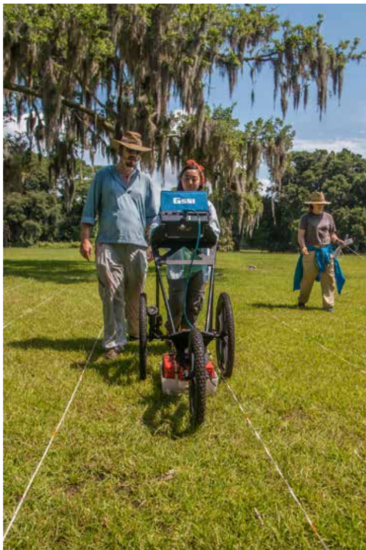
Figure 3: Ground penetrating radar in use at Santa Elena, June 2016. Justin Cramb (left) and Bianca Garcia (right). (Photo by Sandy Dimke, Santa Elena Foundation)
