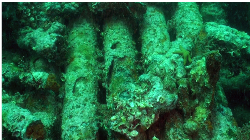
Figure 4: Fire tubes inside the boiler at the wreck of the SS Sherman . (SCIAA image)
