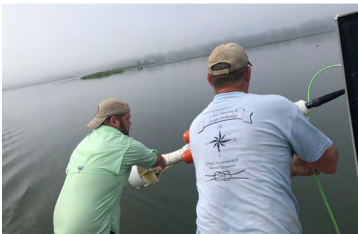
Figure 4: Ryan Bradley and Jim Spirek pitch a cesium magnetometer in the Cooper River for detection of ferrous metals. (SCIAA photo)
