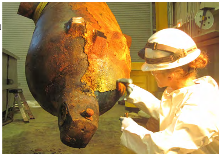
Figure 5: WLCC conservator removing cocoon from exterior of the Dahlgren. (Photo courtesy WLCC)
