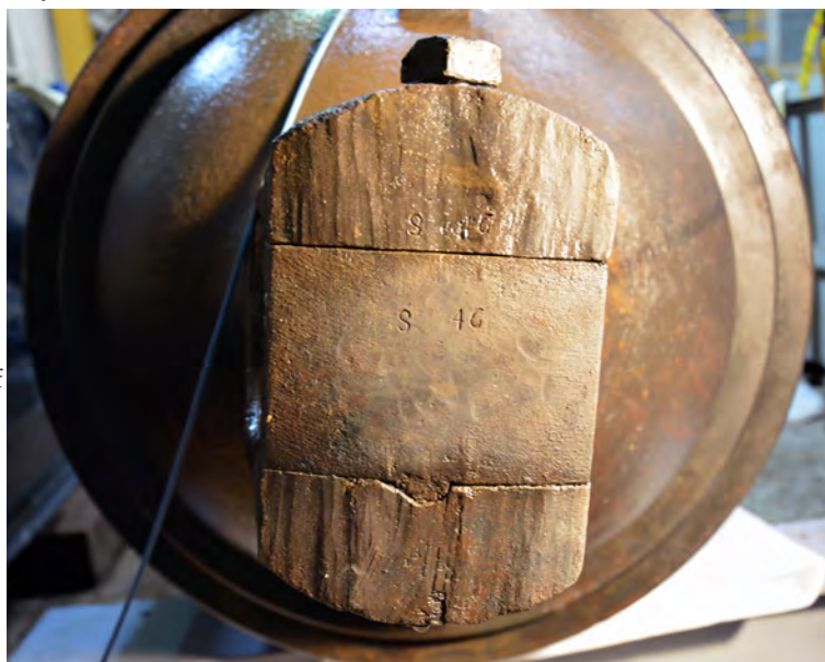
Figure 8: Rear view of VII-inch Brooke cascabel showing upper and lower jaws with block and square-headed pin. Note serial markings on top jaw and block, and groove at lower block and jaw presumably to key the piece in place. (Courtesy WLCC)
