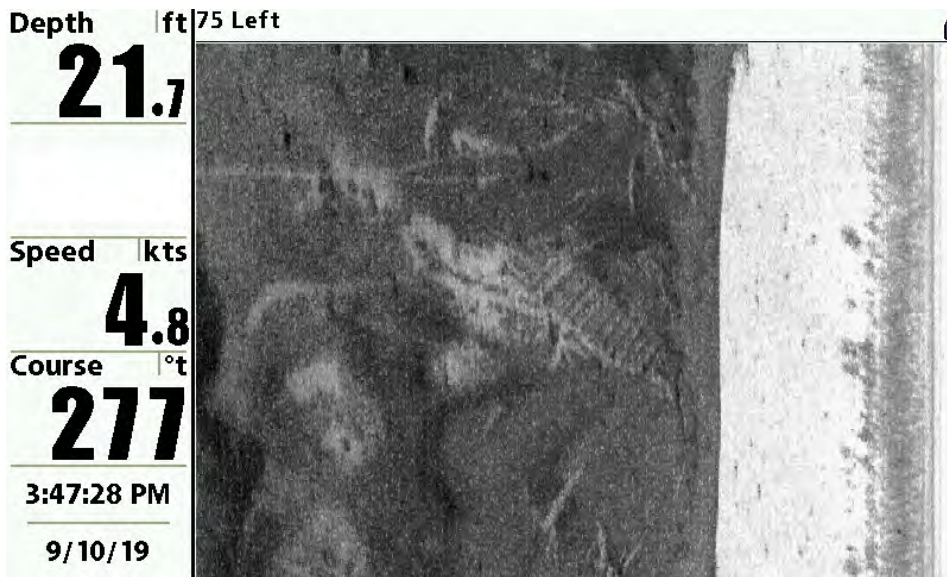
Figure 3: A side scan sonar sonogram shows a shipwreck and other submerged cultural resources in the Cooper River. (SCIAA graphic)
