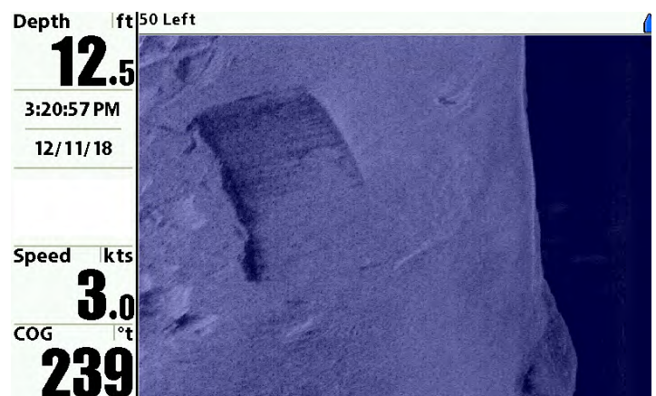
Figure 7: A sonogram of a barge wreck in the Wambaw Creek. (SCIAA graphic)
