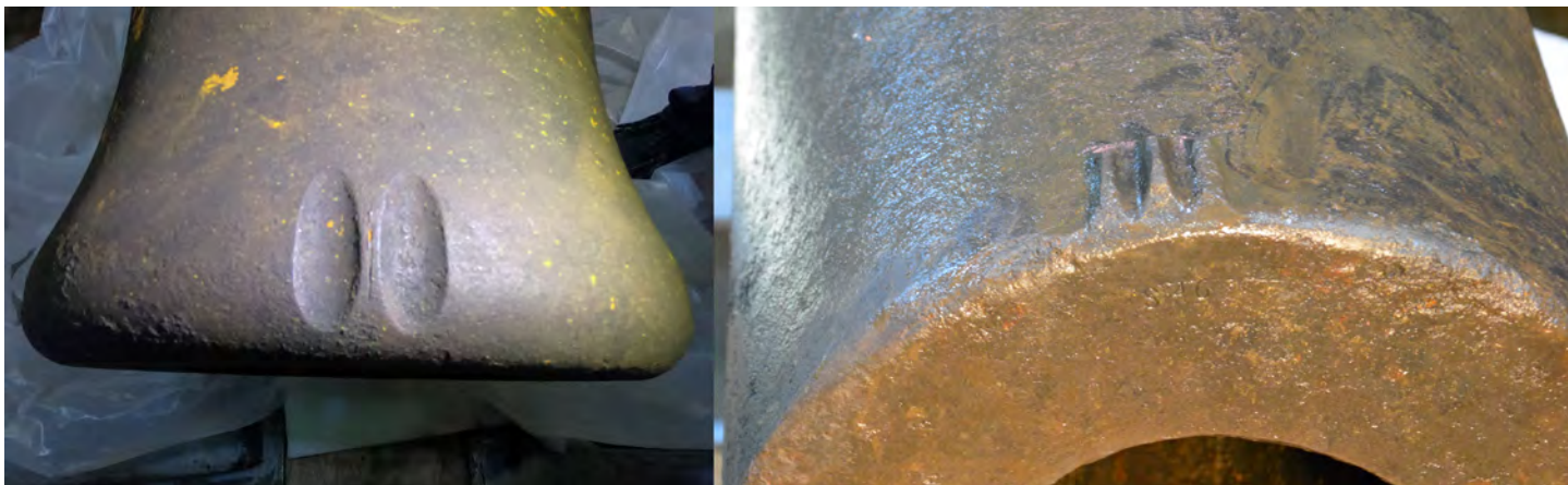
Figure 9: Views of muzzle sights of Dahlgren, on left, and Brooke, on right. (SCIAA and WLCC photo)
